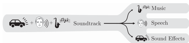
Fig. 1. Illustration of the cocktail fork problem: given a soundtrack consisting of an audio mixture of speech, music, and sound effects, the goal is to separate it into the three corresponding stems.
